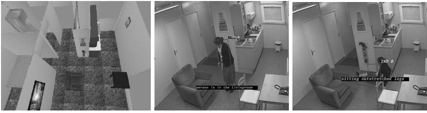
Fig. 5. Recognition of two video events in Gerhome laboratory. (a) 3D visualization of the experimental site “Gerhome”, (b) person is in the livingroom, (c) person is sitting in the floor with outstretched legs.
