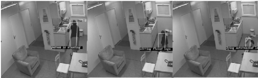
Fig. 8. Recognition of the “falling down” event. (a) person is standing. (b) sitting with flexed legs. (c) lying with outstretched legs.
