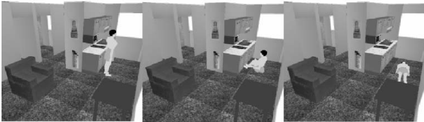
Fig. 9. 3D visualization of the recognition of the “falling down” event. (a) person is standing. (b) sitting with flexed legs. (c) lying with outstretched legs.
